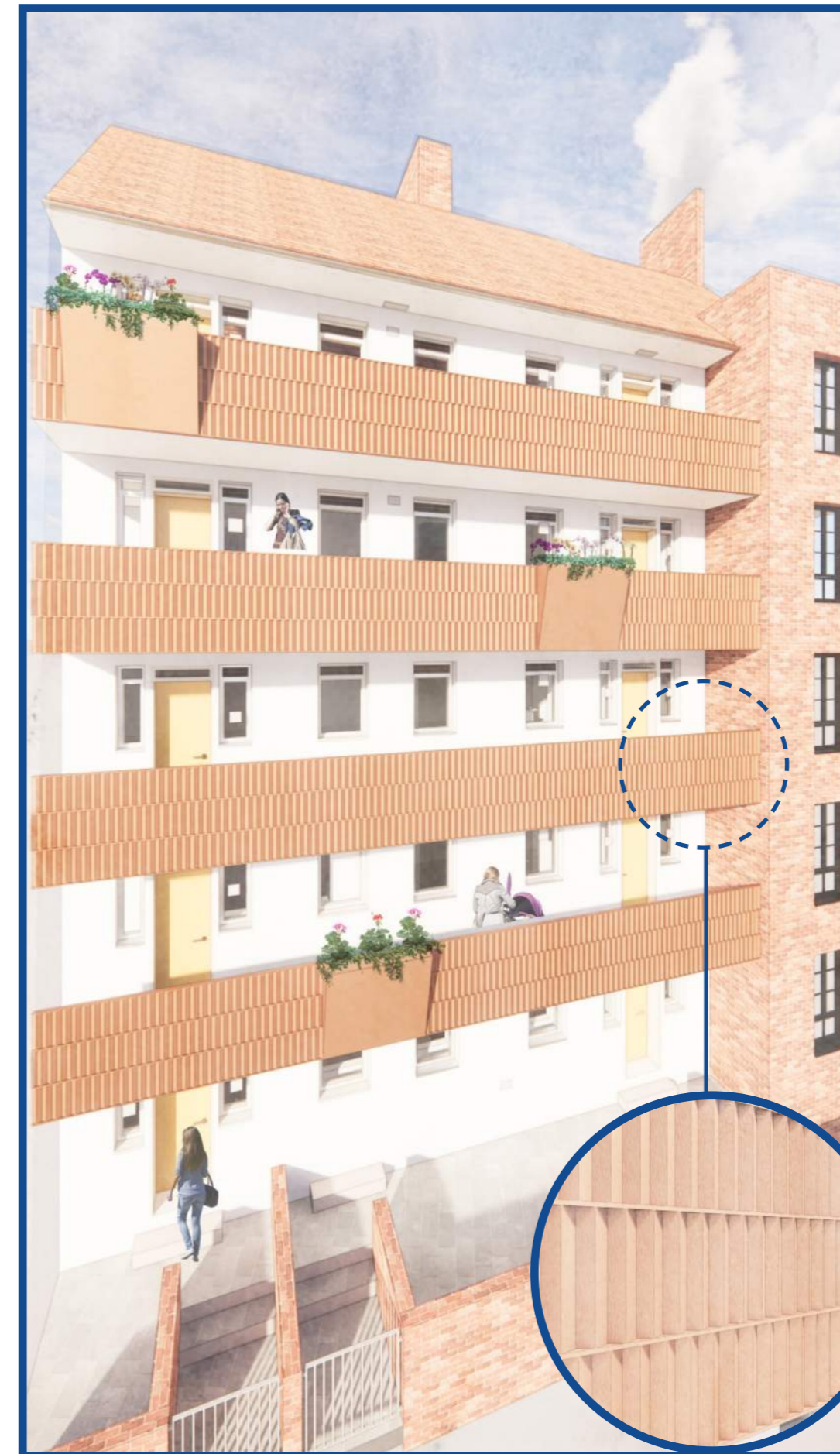
Example metal balustrades
